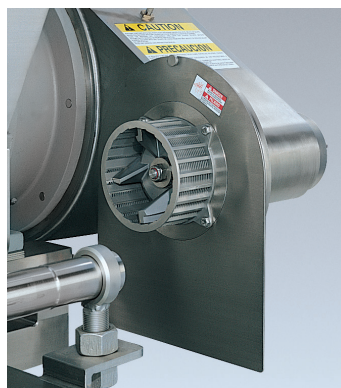
Cutting unit with cutting enclosure removed (for illustration).
